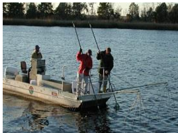
Photo 8.3.6-1. Fyke net positioned in the littoral zone of a Wisconsin lake (right) and an electroshocking boat (left).
